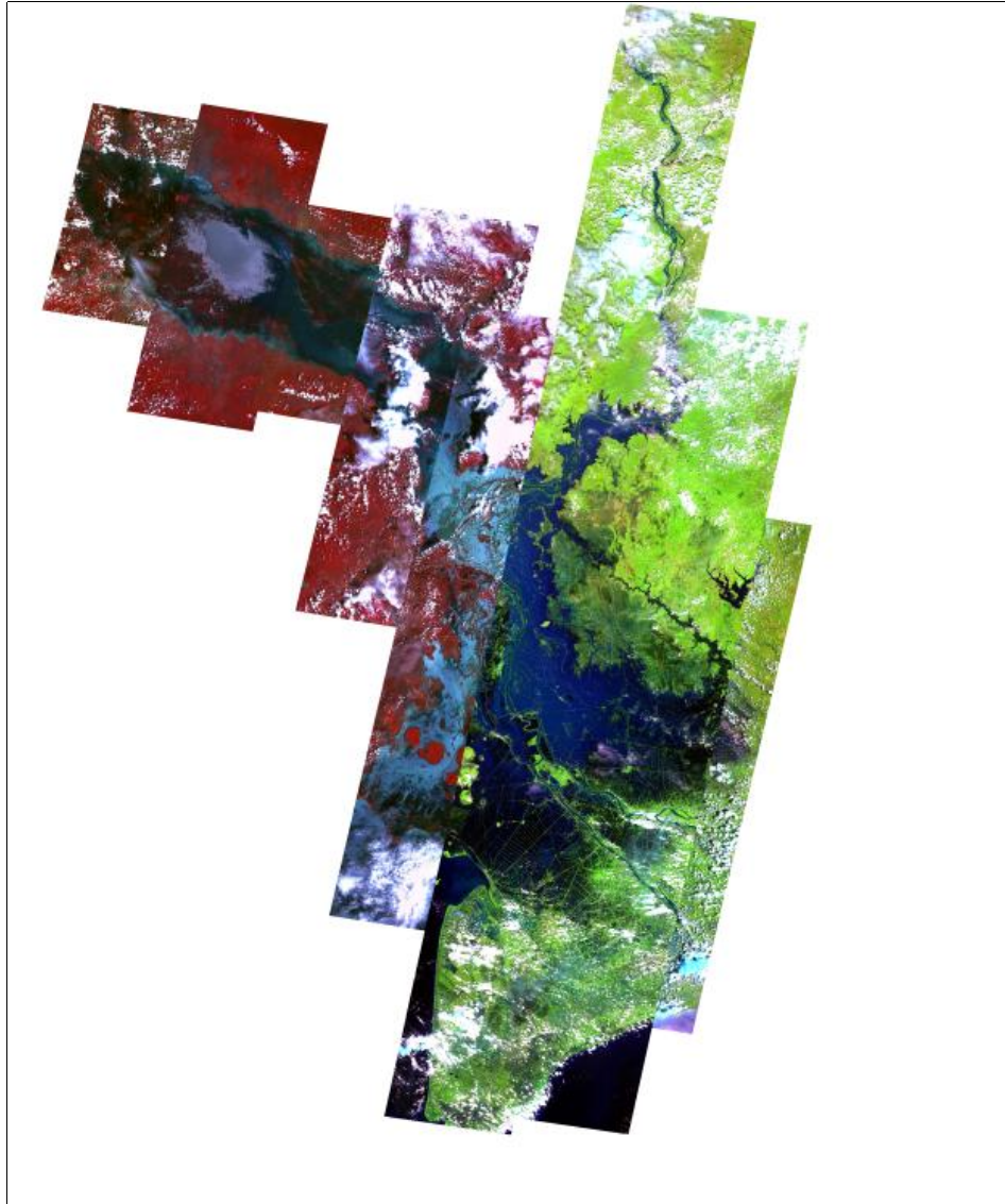
Figure 1: 2000 flood mosaic. The strips on the right were composed from SPOT 4 scenes (R: band 4, G: band 3, B: band 2) while the strips on the left were composed from SPOT 1 and SPOT 2 scenes (R: band 4, G: band 3, B: band 2).
