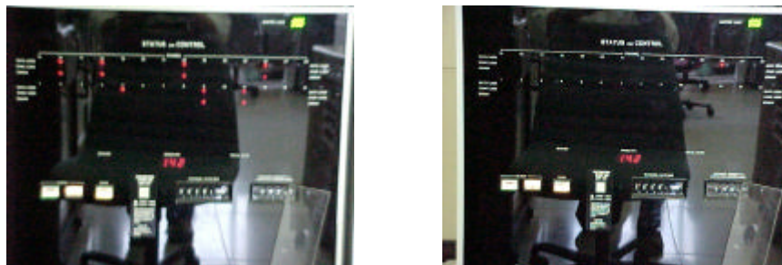
Figure 5: Data Processing System/HDDR (Left: Red Light shows Sync Loss, Right: Normal scenario)
