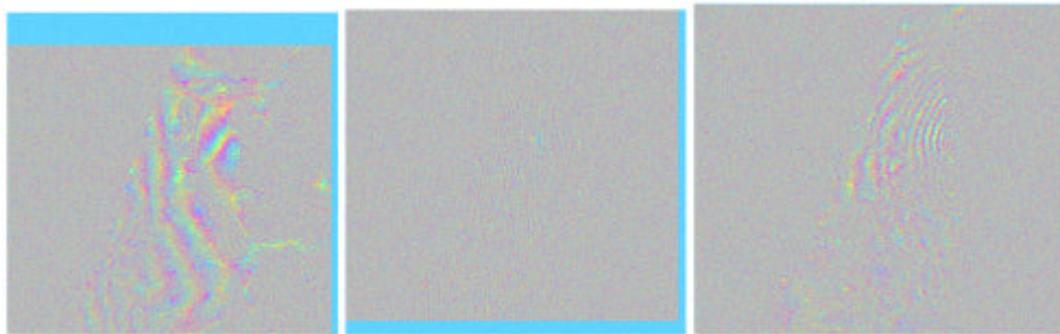
Figure 4. Three inteferograms: May 06/Jan. 21 (left, B_{\perp} \cong 97\text{m} ), May 06/Sep. 23 (middle, B_{\perp} \cong -220\text{m} ), May 06/Oct. 28 (right, B_{\perp} \cong 5\text{m} ), where B_{\perp} denotes the perpendicular baseline.
