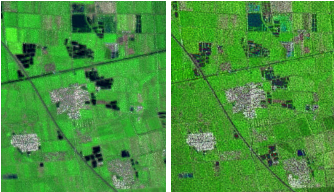
Figure 2 HIS fused TM and SAR images. Figure 3 Brovey fused TM and SAR images RGB – TM bands 7 4 3 and Intensity – SAR R G B – TM bands 7 3 4 and Intensity – SAR
