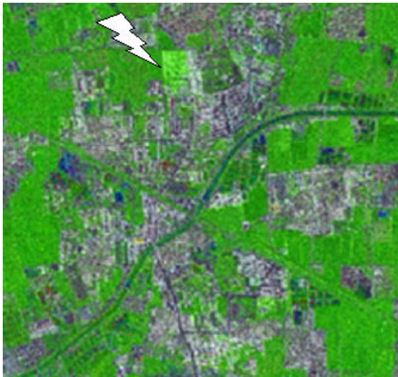
Figure 4. HIS fused TM and SAR images RGB – TM bands 7 4 3 and Intensity – SAR shown land patches( low green)
