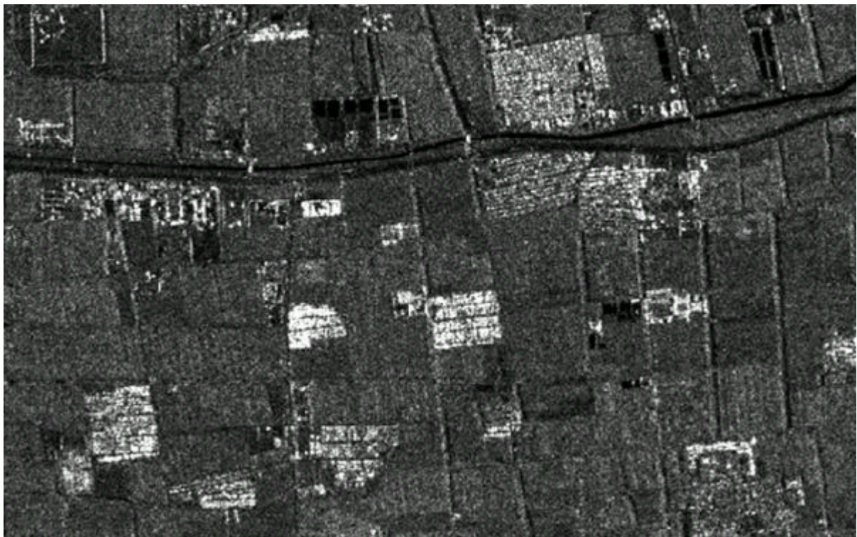
Figure 1 Enhanced Radar SAR image by edge enhancement filtering. Window size was 5x5.
