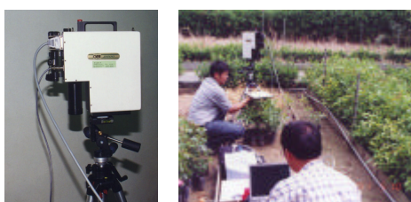
Figure 2. The configuration of the spectroradiometer and components setup for field spectral measurements
