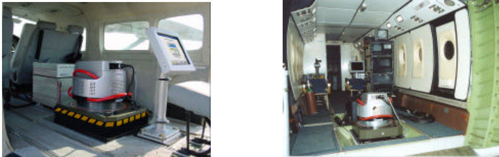
Figure 4. From left to right: installation in a Cessna 208B Caravan in Japan; installation in a CASA 212 in Italy.
