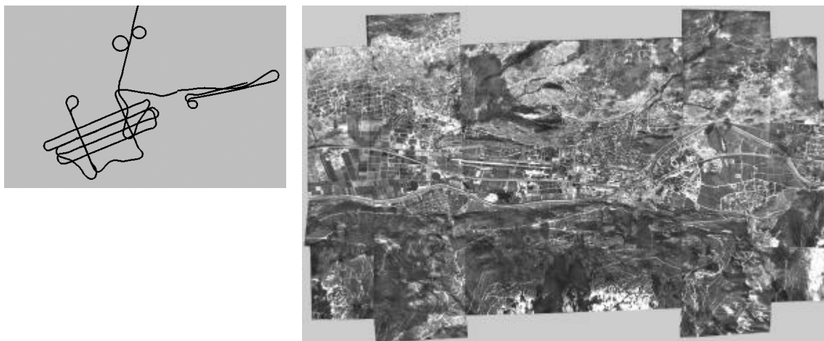
Figure 5: From left to right: Sion block flight path, in-flight IMU alignment loops and double line flown in opposed directions to correct for IMU misalignment. The results of such a flight are perfectly parallel flight lines, as seen in the superimposed rectified strip imagery of the Sion block.
