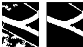
Figure 3. Illustration of the result after image-processing (a) Redundant Noise Reducing (b) Road-region Recognizing
