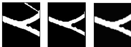
Figure 4. Illustration of the result after image-processing (a) Road-region Recognizing (b) PART(A) of The Pattern of Roads Refining (c) PART(B) of The Pattern of Roads Refining
