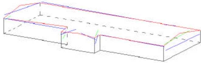
Fig.9 Detected Lines for outline of gable roof
