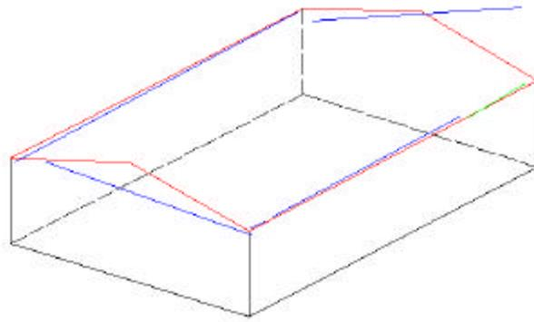
Fig. 10a and 10b the possible error lines of gable roof caused by Hough Transform
