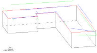
Fig.8 Detected lines for outline of plane roof
