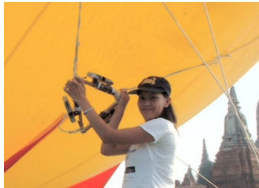
Figure 6: camera mount system with off-nadir looks angles
