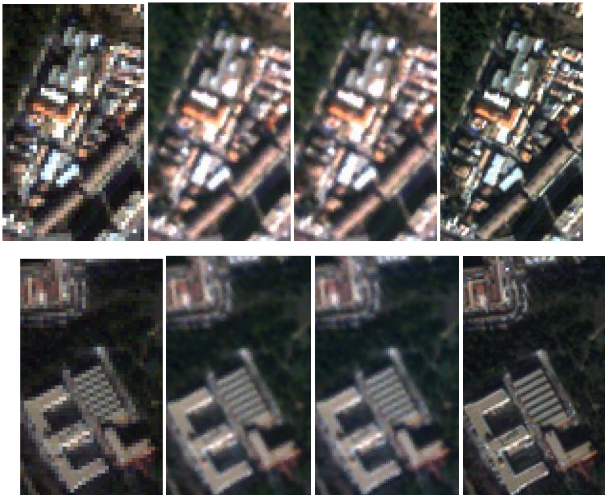
Figure 3: Results of applying SRVPLR and SRASW to a set of simulated QuickBird images. From left to right: a) One of the 9 input 4.8m pixel LR images. b) SRVPLR 2.4m pixel result. c) SRASW 2.4m pixel result and d) Original 2.4m true image.
