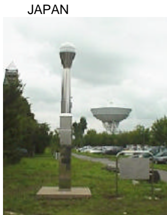
Figure.3. GPS continuous observation station
