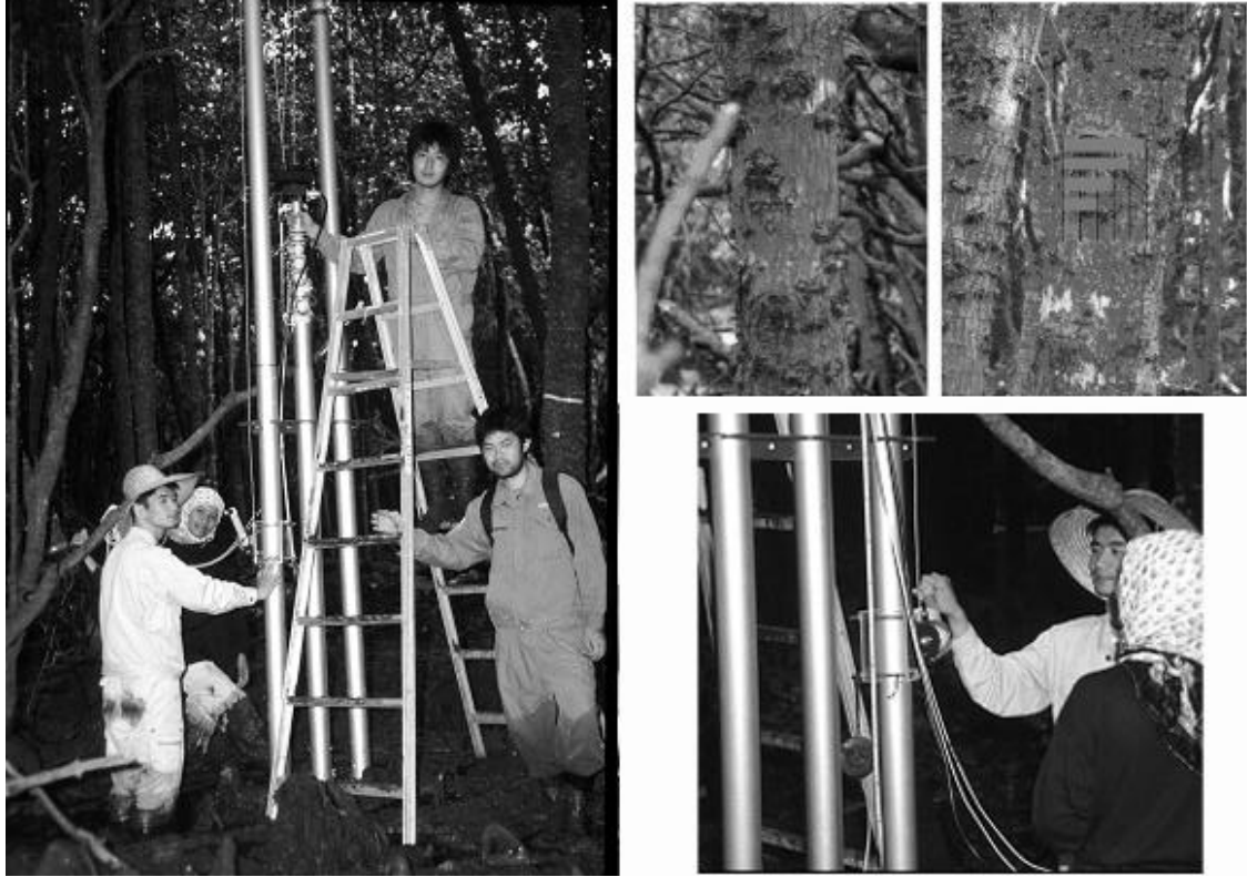
Fig. 2 Setting of new pole system in a mangrove stand (left), operation of the handle reel (below right), a taken imagery of a trunk and drawn scales on an imagery of a trunk with an image processing software (above right)
