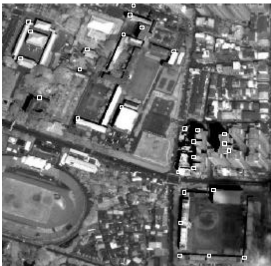
Figure 9. Generated True Orthoimage and Check Points
