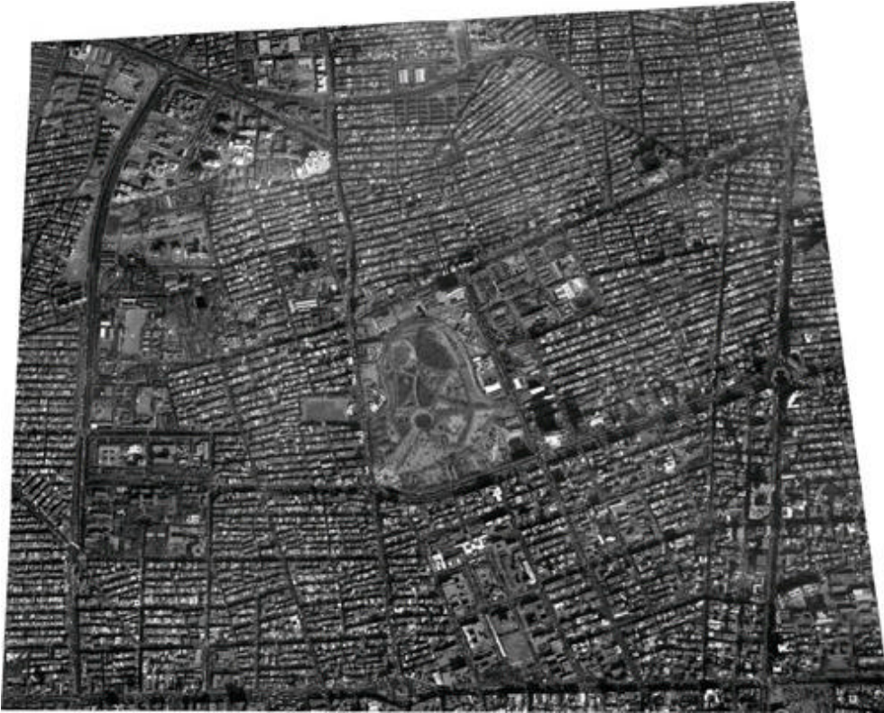
fig 7-Orthoimage that correct by DLT method with geopic software
