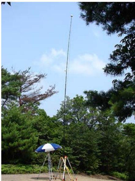
Fig. 5 The GPS pole slightly leaned when used for GPS measurement at K2.
