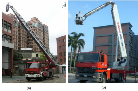
Figure 2. Two main types of ladder trucks: (a) turntable ladder and (b) aerial ladder platform.
