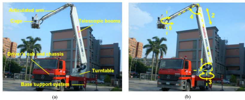
Figure 3. (a) Components of a ladder truck and (b) rotation and translation of a ladder.
