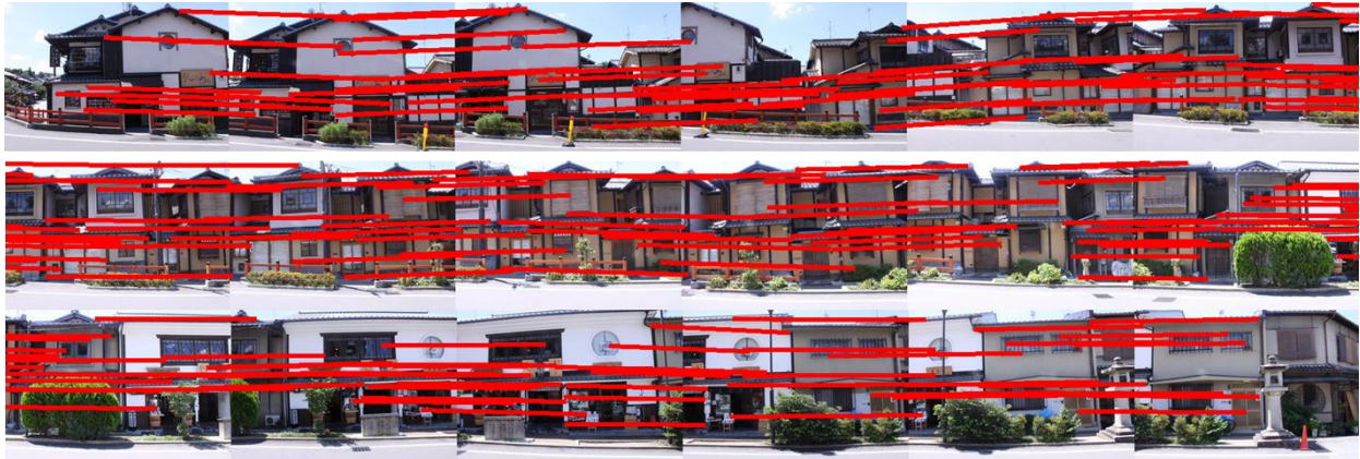
Figure 6 Passpoints of 17 successive stereo-pairs selected automatically using proposed method
