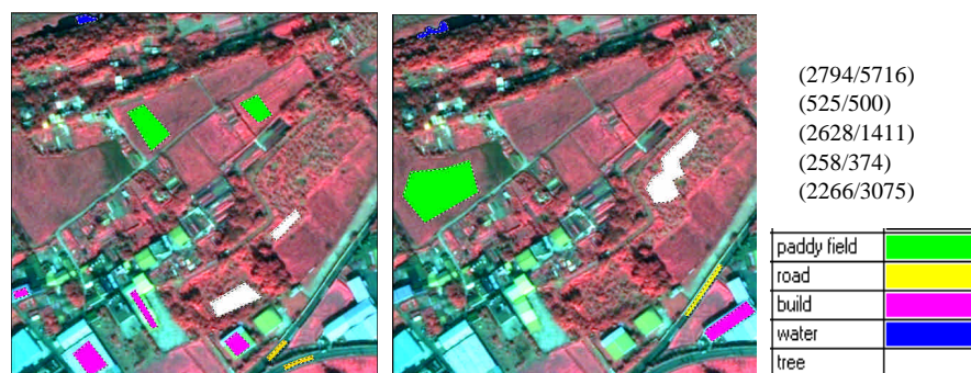
Figure 2 Training and testing area location show on data set. The number of training and testing samples for each class are shown in parenthesis at the legend.
