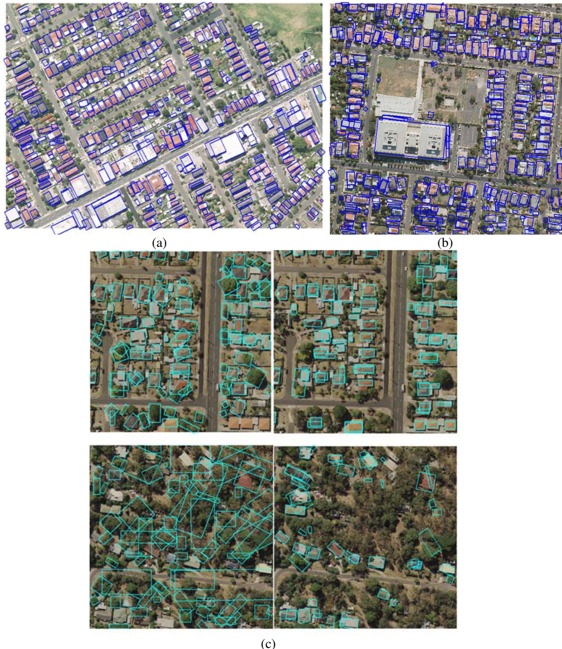
Fig. 3. Separation of trees and buildings for building detection in (a) Fairfield, (b) Moonee Ponds and (c) Knox. In (c), the detected buildings by Awrangjeb et al. (2010) on two samples are shown in left for comparison, while the detected buildings with the methods described here are presented on the right.
