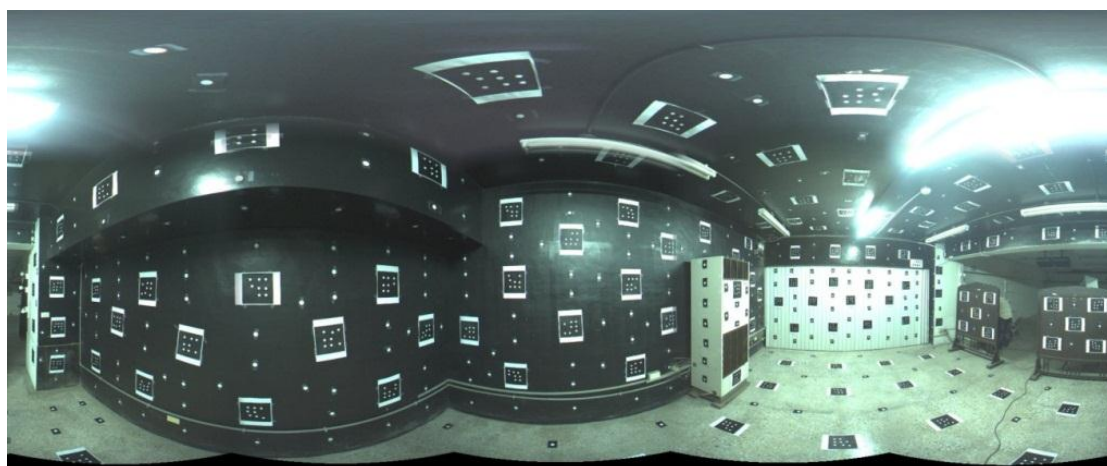
Fig. 4. The panoramic view of calibration field taken by Ladybug3.
