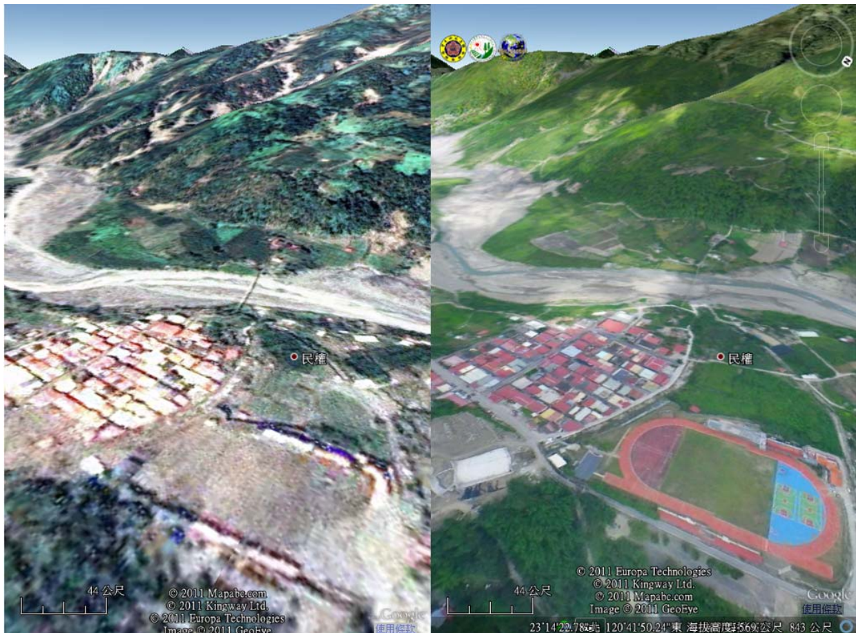
Figure 9. The screen shot of (a) Formosat-2 image (2m) and (b) UAV image (25cm) published on Multistage Remote Sensing Geospatial Information System ( http://geodac.ncku.edu.tw/swcb/multistage.aspx ).
