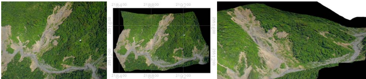
Figure 6. One example of (a) the original photo taken at Laonung area, (b) the orthorectified photo, and (c) the orthorectified photo overlaid on DTM.
