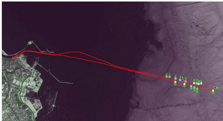
Figure 14. Trajectories and points of sea ice thickness measurement overlaid on RSI image. (Feb.22, 2011)
