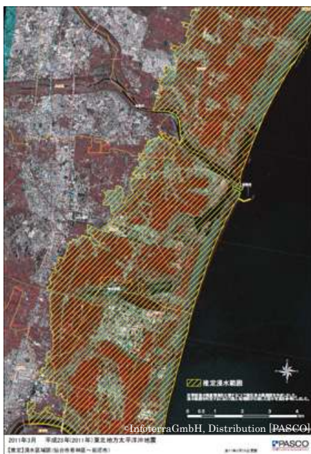
Fig3.Rapid mapping of flood by TerraSAR-X
