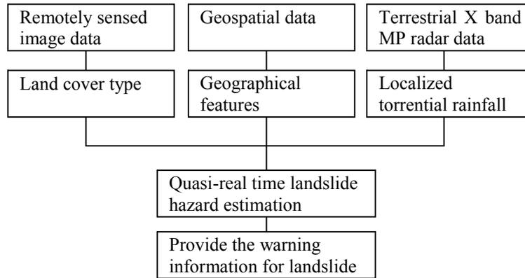
Figure 3: A concept of warning system for landslide disaster.
