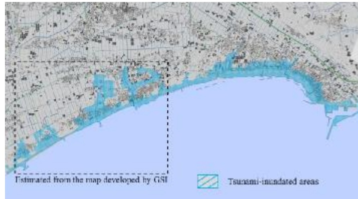
Figure 6: Final estimates of tsunami-inundated areas in Asahi City, Chiba Prefecture, after the 2011 off the Pacific coast of Tohoku Earthquake
