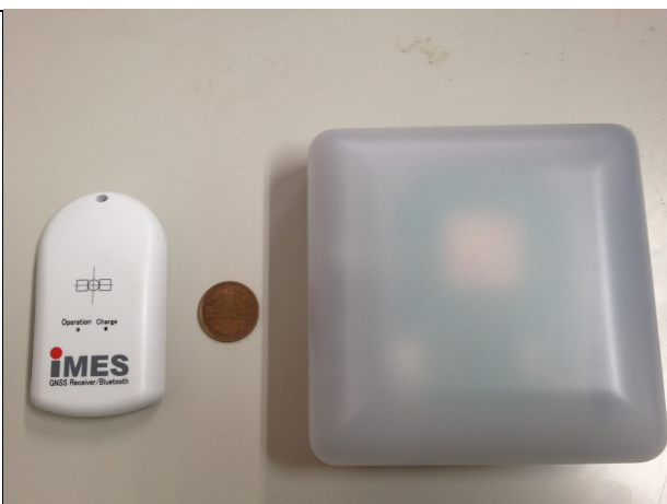
Figure 2: IMES receiver and transmitter
