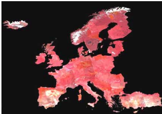
Fig.8 DMC complete mosaic of Europe at 32m GSD acquired within a window of four months (2007)
