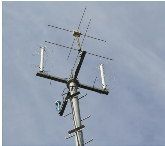
Figure 4: Turnstile antenna and Quadrifilar helix antenna.
