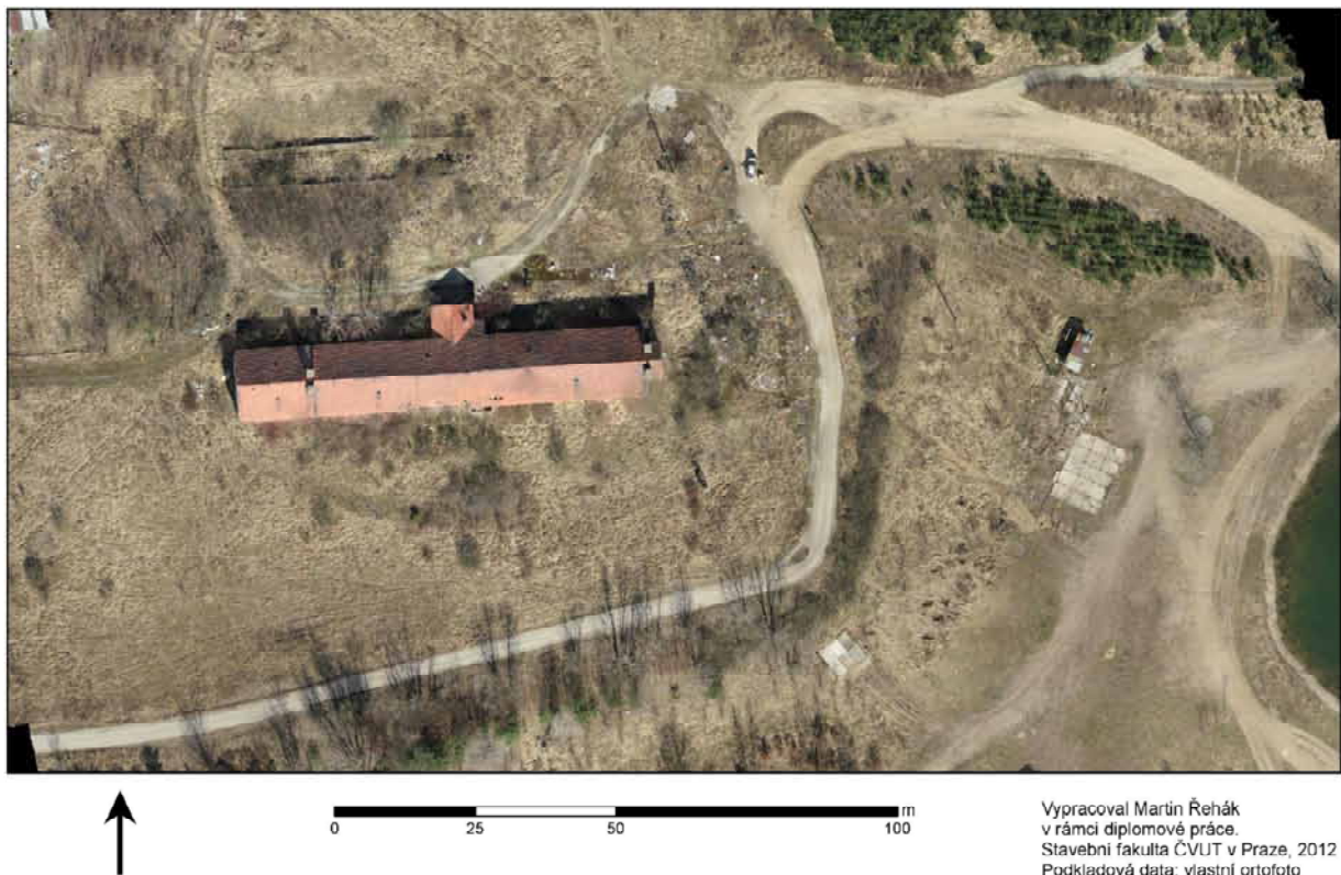
Figure 5 : Orthophoto taken from UAV Mikrokopter; software Aerogis, pixel size 3cm, 103 images (6 ha). RMS of about 4cm (this value was computed from GPS measured checkpoints, which are not used in computing/adjustment). Approximate time of preparation and processing: 8 hours.
