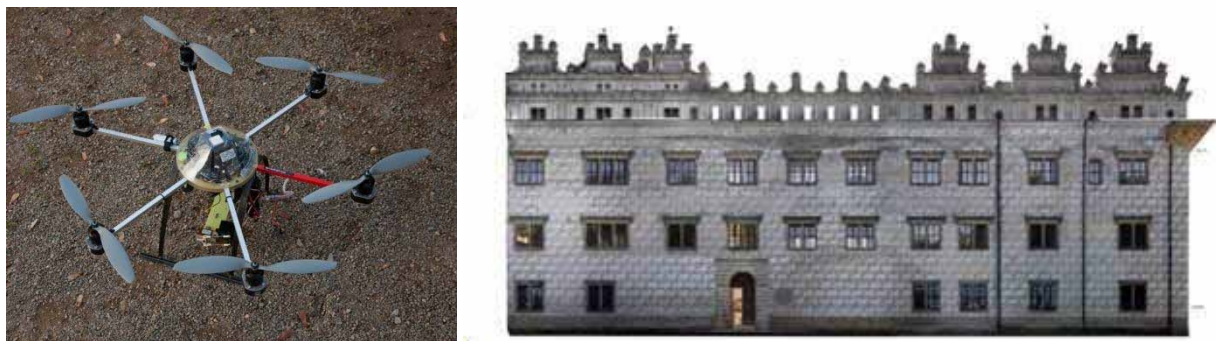
Figure 1 : Hexa-copter with sophisticated electronic parts (left), final photo plan of the north part of the Litomyšl castle consisting of images taken from hexa-copter equipped with compact camera Canon S100 and from hand held camera Canon 5D
