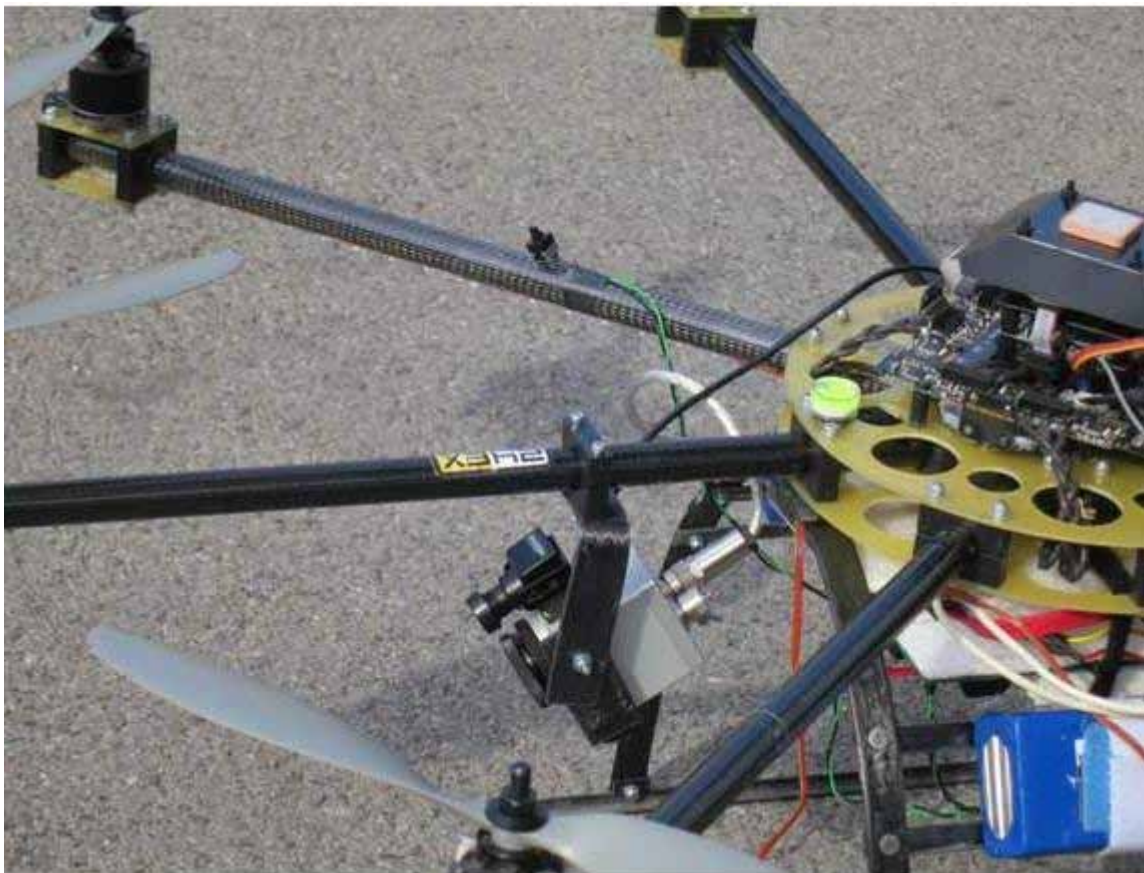
Figure 6 : Detailed view of thermal camera and small surveillance camera, max load capacity 1,5 kg.
