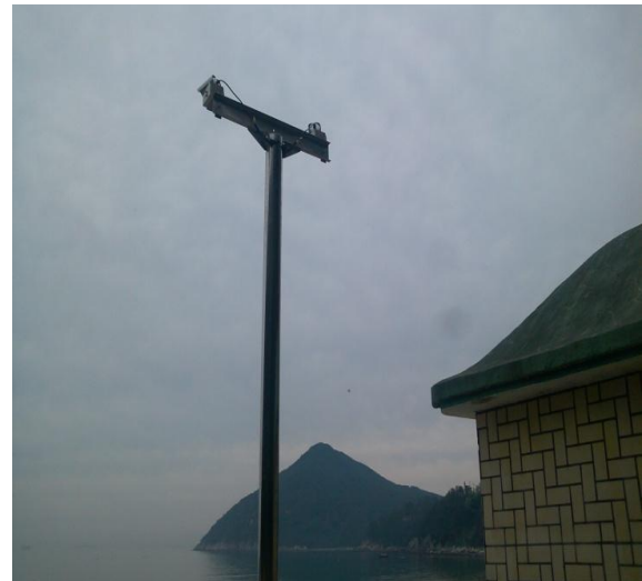
Figure 2: Network Camera for beach litter monitoring.
