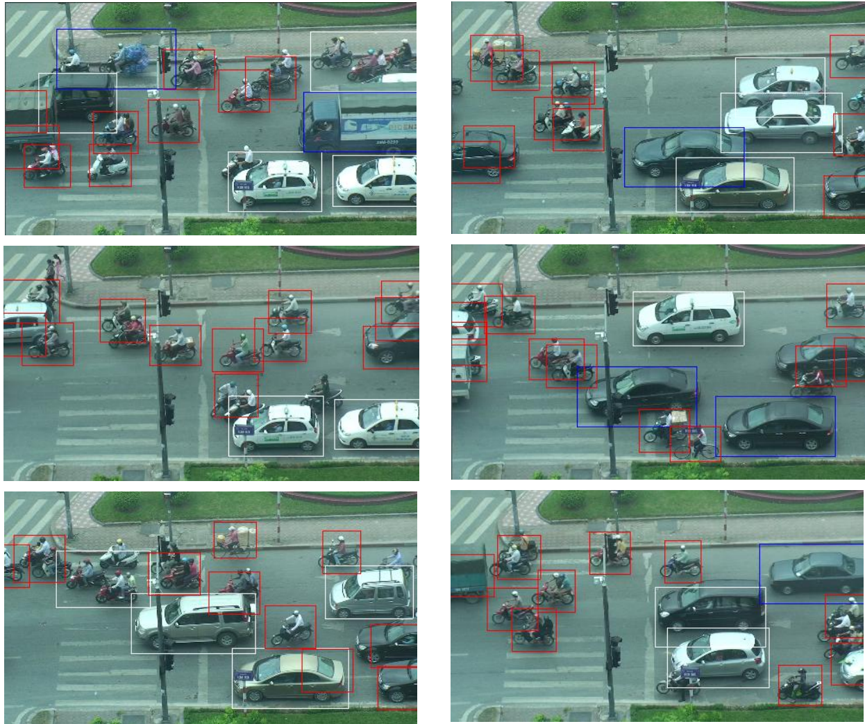
Figure 9: Results of vehicle detection. While box denotes bright car, blue box denotes dark car, and red box denotes motorcycle.
