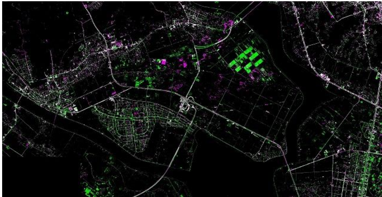
Figure 2 Extraction of jetted sand areas on the roads by overlaying two GeoEye-1 images
