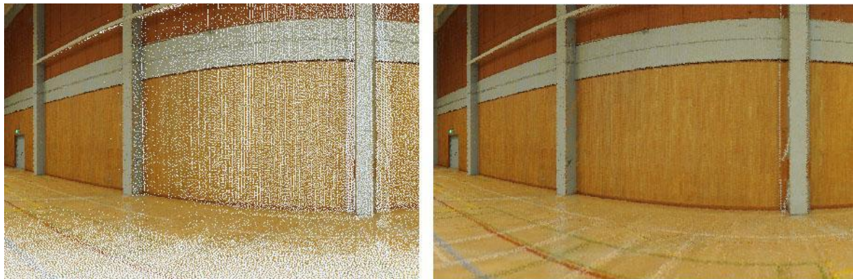
Figure 2: Part of a panoramic image in which the left image is the result after a viewpoint translation of 6 m the sensor point and the right image is the result after filtering
