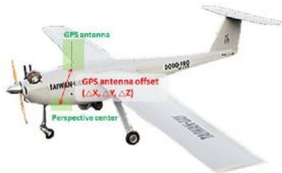
Figure 3: the offset between the GPS antenna center and the camera perspective center
