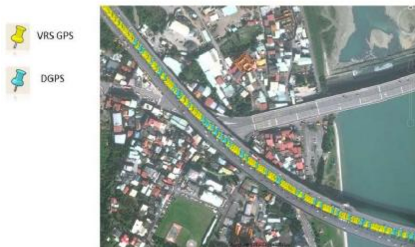
Figure 12: Part of L1/L2 DGPS and VRS GPS positioning results overlay on the Google Earth
