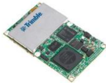
Figure 5: Trimble BD970 GNSS OEM board
