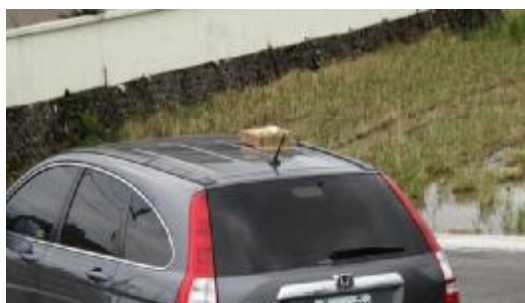
Figure 6: GPS antenna attached on the top of the vehicle
