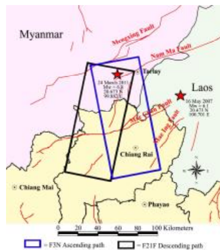
Figure 3: Location map of left-lateral fault system in the Golden Triangle area and footprint of Radarsat-2 SAR imagery both in ascending and descending orbits.
