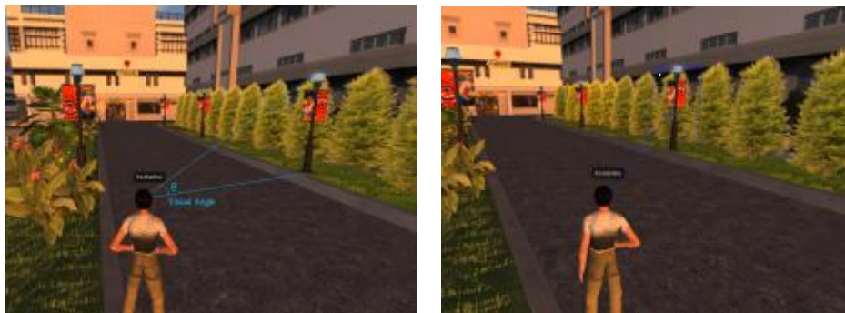
Figure 6: Left: Meaning of visual angle (vertical); Right: Extraction method of visual angle in OpenSim, by using the method of bounding box, and calculate the visual angle for a box in horizontal and vertical direction.
