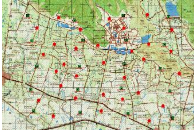
Figure 3 Ground control points and check points on the study area
