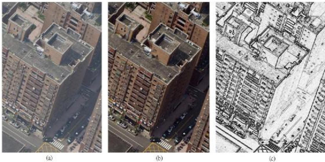
Figure 4: (a) Original image; (b) Image after enhancement; (c) Edge map extracted from the original image
