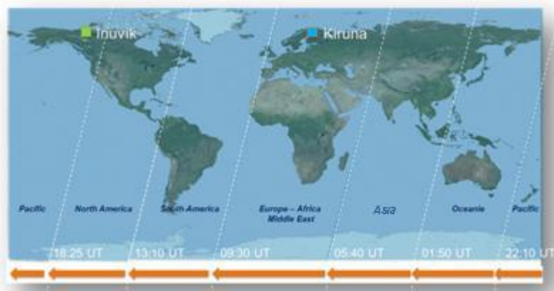
Figure 2: Two polar stations, located in Inuvik and Kiruna, are used to uplink the 6 daily tasking plans related to the 6 zones: Pacific, Japan/Oceania, Asia, Middle East/Europe/Africa, South America, North America. © Astrium Services / Spot Image 2011
