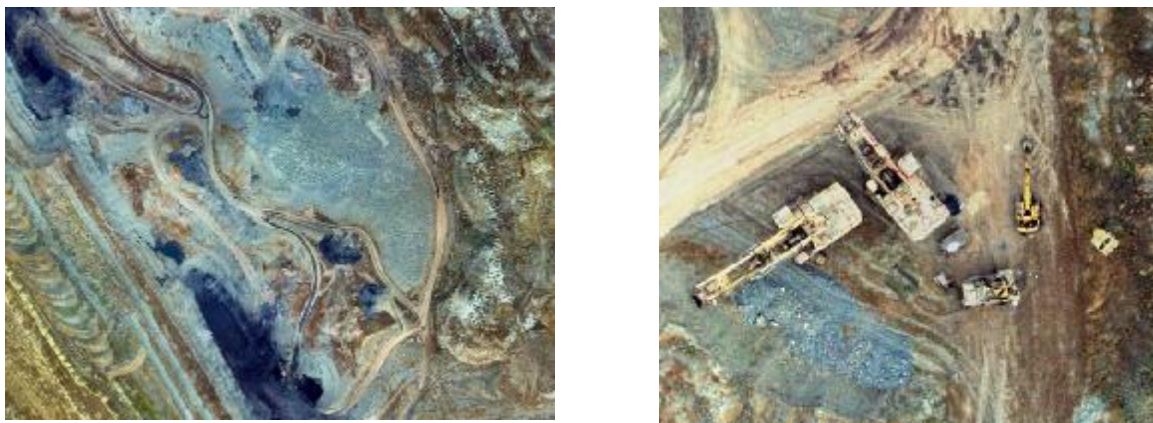
Figure 5: Orthomosaics generated from drone photos; scales 1:5000 (left) and 1:500 (right).
