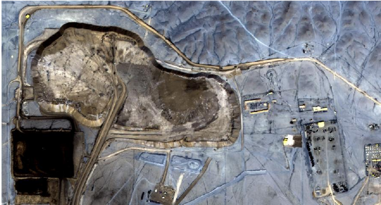
Figure 4: Pan-sharpened 8 bands stereo HRI as basis for topographic and thematic mapping.
