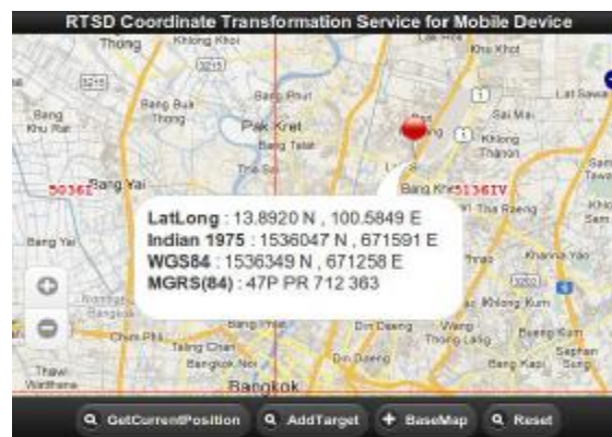
Figure 4: Coordinates which are transformed by application is shown in the pop-up block.
