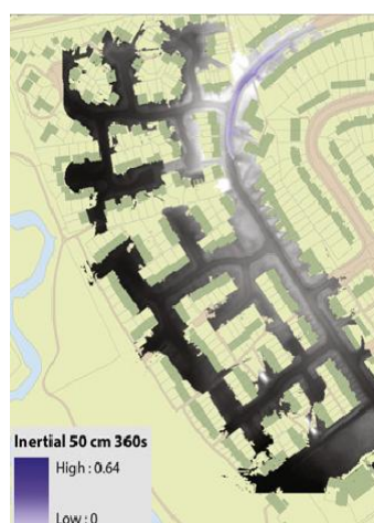
Figure 3 Applying 2D GIS to the water storage estimation models (Fewtrell T. J. et al, 2011).
