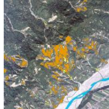
Figure 16: Final landslide areas
