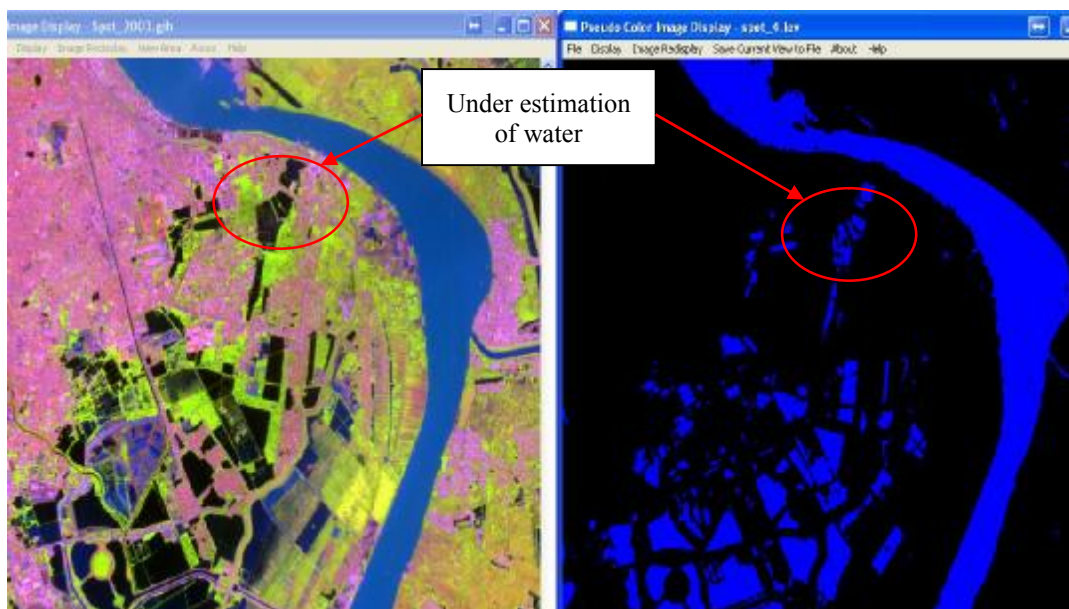
Figure 6: Spot 5 colour composite image (left) and water extraction by level slicing of SWIR band (right)
