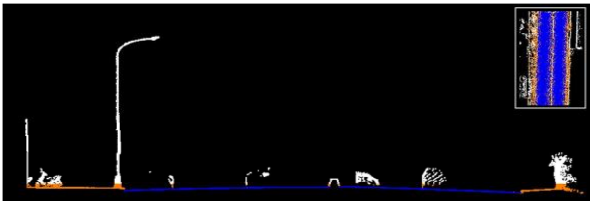
Figure 5: The result of the road point in a profile
