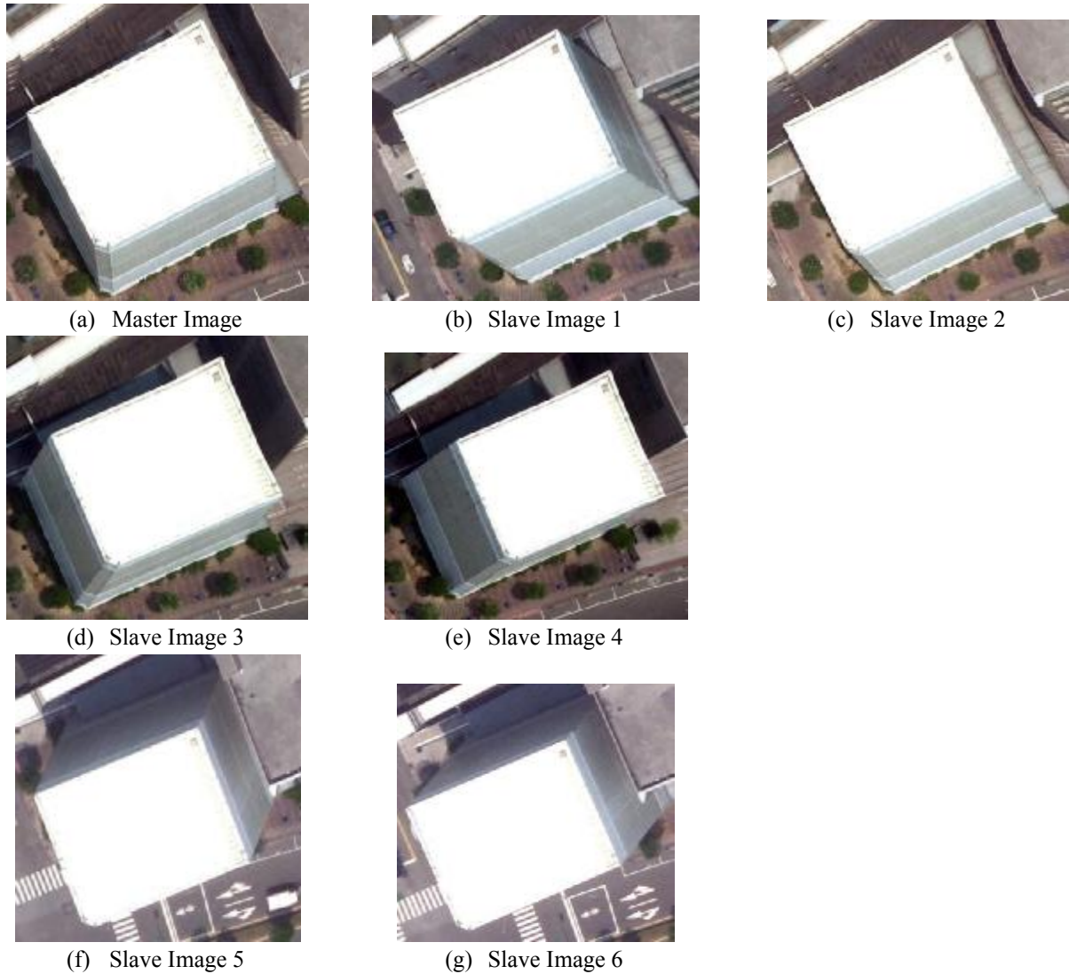
Figure 8: The target building on multiple images with double strips in Case 2, (a) to (e) are the first strip images, (f) and (g) are the second strip images.
