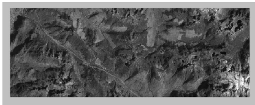
Figure 3.10 Decompressed image when SEB occurs at the 3000 th bit.
