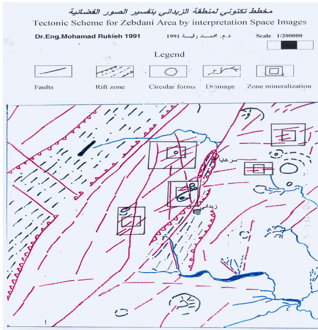
Fig.5- tectonic scheme with zone (hydrothermal Fe- Zn-Cu mineralization) in Zebdani-sirghaya area-Syria by interpretation space images( Rukieh 1991-2003 )
