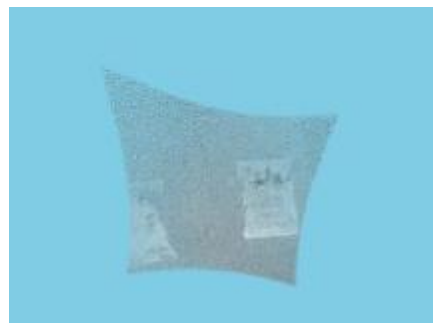
Figure 6: Point cloud data taken with the Time of Flight camera (a bird view)
