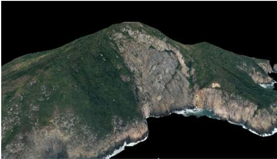
Figure 5: Ortho-photos aerial photos draping over DTM to create a 3-D image
